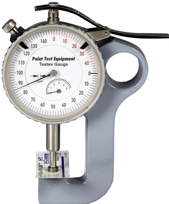
Testex Tape is able to produce accurate replicas on surface temperatures of  $-10$  to  $+65^{\circ}\text{C}$ .
